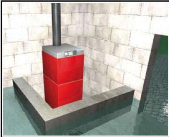
Example of protection of sensitive installations by means of a watertight device
